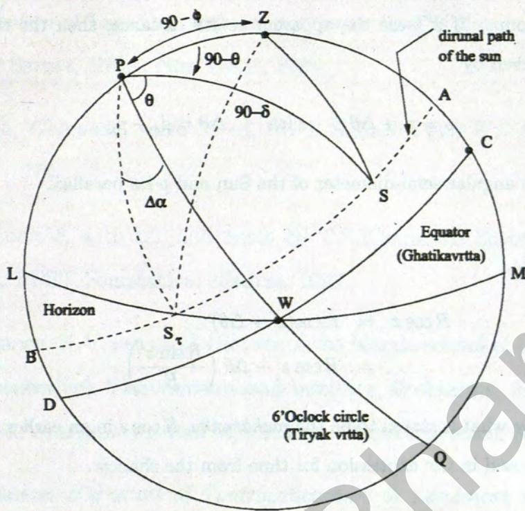
**Fig.5:** Determination of time from shadow measurements.
