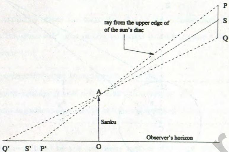
Fig.3: Sectional view of the sun and the shadow of the *Sanku* generated by it.
