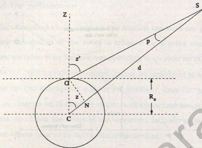
**Fig.4:** The effect of parallax on the measurement of latitude of the observer
